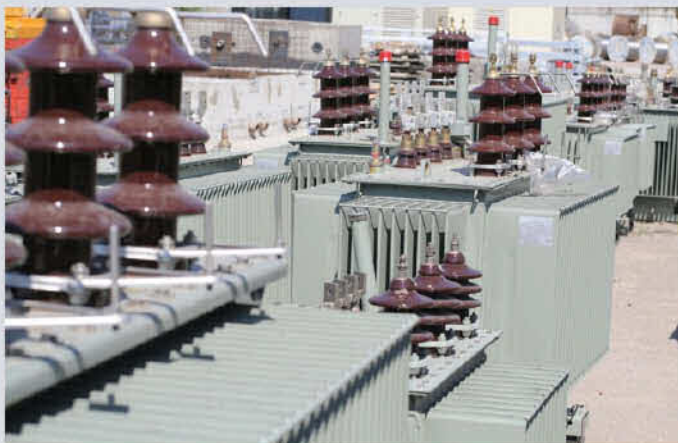
Pole mounted 200kva transformers awaiting collection
